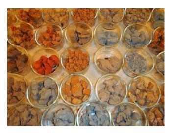
Separate different soils with different sized sieves. Compare the masses of the different particles collected through each sieve. Add the masses of separated matter to see if it weighs the same as the original soil before sifting. Compare the amounts of each type of matters sieved from each soil type.
